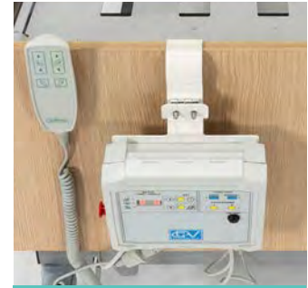
The programmable control box.
